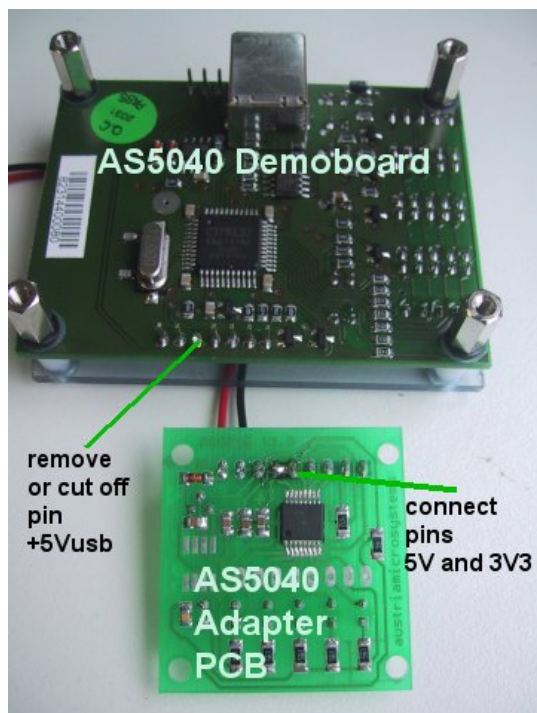
Figure 15: Configuring the adapter PCB for 3.3V operation
