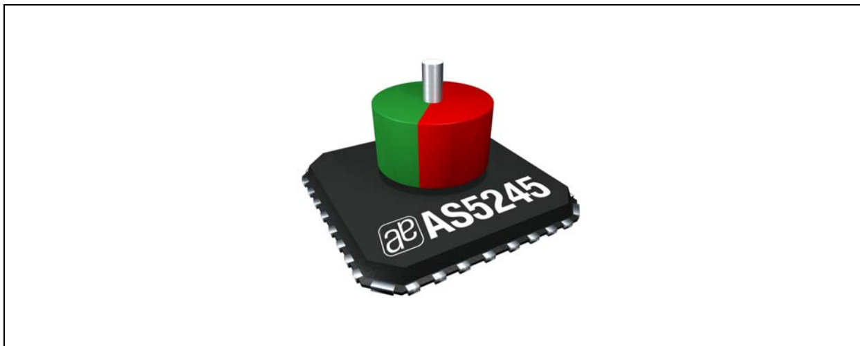
Figure 4. Typical Arrangement of AS5245 and Magnet
